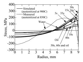
Fig. 2 Circumferential Stress Distribution in SUJ2 Bearing Steel Specimens
