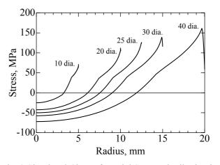
Fig. 3 Simulated Circumferential Stress Distribution in SKS3 Tool Steel Specimens
