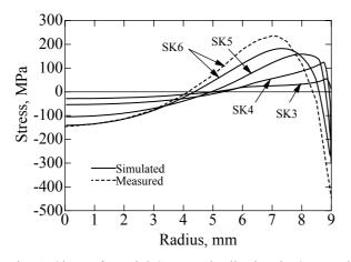
Fig. 1 Circumferential Stress Distribution in SK Tool Steel Specimens
