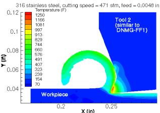
**Figure 2:** Predicted temperature distributions using Third Wave  $AdvantEdge^{TM}$ . The plots show that the tool/chip interface temperature is comparable when cutting with these two inserts.
