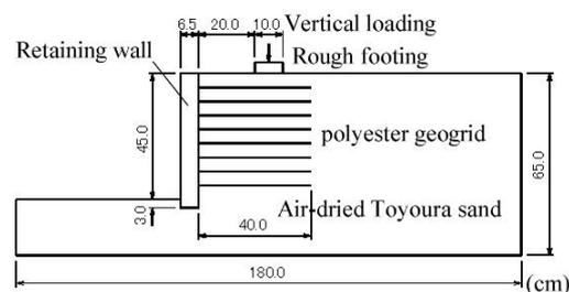
Fig.1 Physical model test
