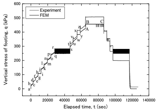
Fig.4 Observed and computed time histories of footing pressure
