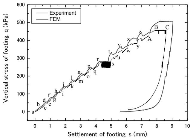
Fig.3 Observed and computed footing pressure-settlement relations
