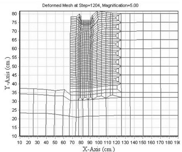
Fig.6 Computed ground deformation
