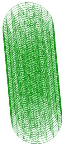
Figure 19: Structured hexahedral mesh of the cylinder
