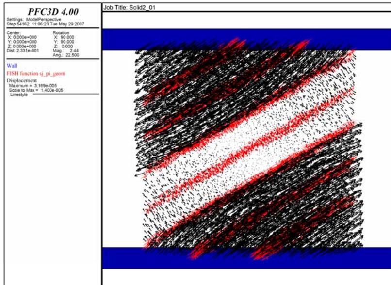
Figure 16 Displacement field in the PFC3D specimen at axial strain of 0.05%
