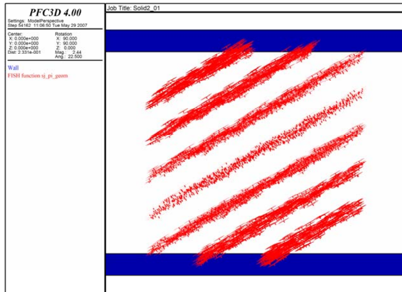
Figure 14 PFC3D specimen after insertion of the seven joints (consisting of 5419 smooth-joint contacts)
