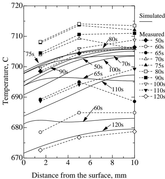
Fig.5 Measured and Simulated Temperature Distributions during Air-cooling.
