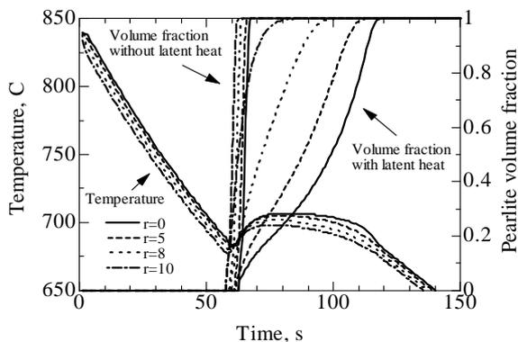
Fig.6 Temperature and Pearlite Volume Fraction Predictions in Air-Cooled Cylinder.
