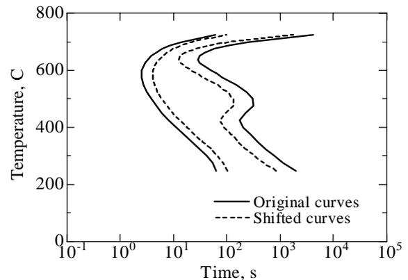
Fig.3 Original and Shifted TTT Curves of 52100 Bearing Steel.
