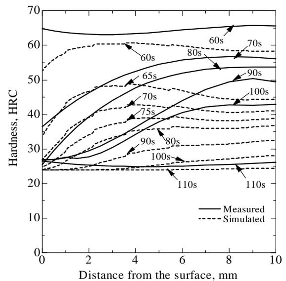
Fig.9 Experimental and Simulated Hardness Distributions in Specimens.
