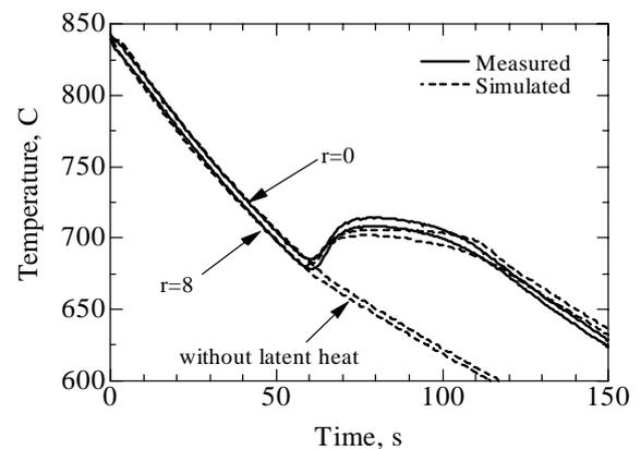
Fig.4 Measured and Simulated Cooling Curves during Air-cooling.
