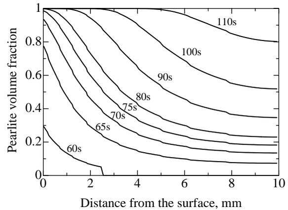
Fig.7 Simulated Distributions of Pearlite Volume Fraction in Air-Cooled Cylinder.
