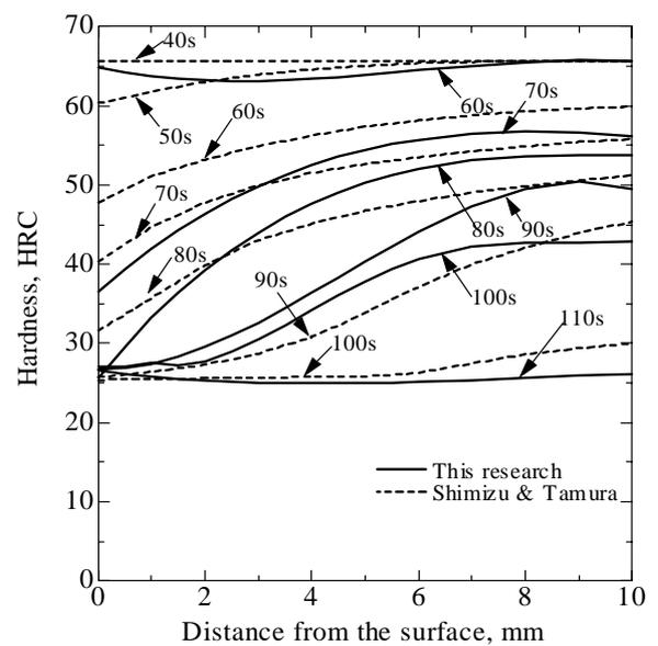
Fig.2 Measured Hardness Distribution in Specimens.
