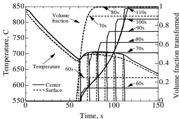
Fig.8 Temperature and Pearlite Volume Fraction Predictions in Air and Brine-Cooled Cylinder.
