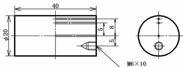
Fig.1 Test specimen Dimensions and Location of Instrumented Thermocouple Holes.
