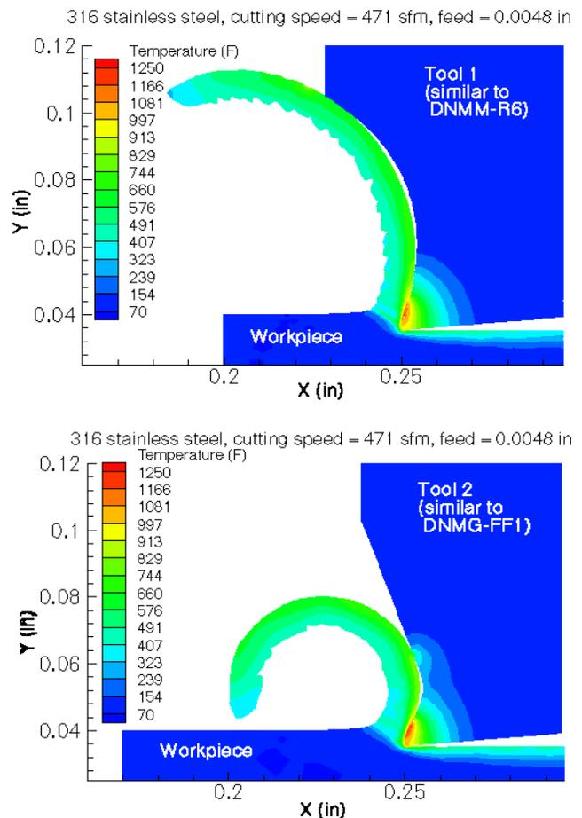
**Figure 2:** Predicted temperature distributions using Third Wave *AdvantEdge™*. The plots show that the tool/chip interface temperature is comparable when cutting with these two inserts.
