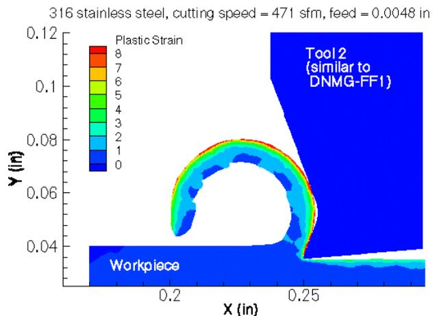
**Figure 1:** Two inserts are modeled and compared under identical process conditions. Predicted plastic strain in chip and workpiece material is shown. The plastic strain on the back of the chip formed by Insert 2 is higher than that formed by Insert 1, indicating Insert 2 can break chip more effectively.
