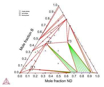
Figure 9: Calculated Fe-Nd-B isothermal section at 1173 K with experimental data from [1985Bus] and [1986Bus].
