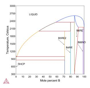
Figure 7: Calculated Nd-B phase diagram.
