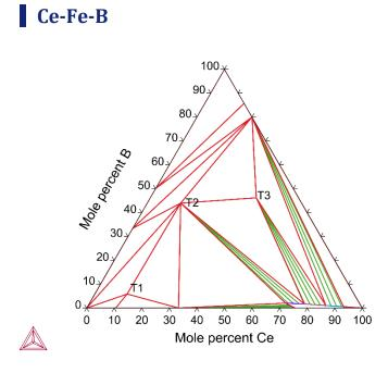
Figure 11: Calculated Ce-Fe-B isothermal section at 973 K.
