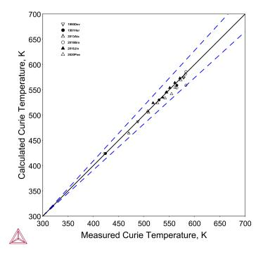
Figure 3: Comparison of calculated vs experimental Curie temperatures.
