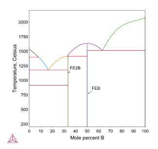
Figure 5: Calculated Fe-B phase diagram.
