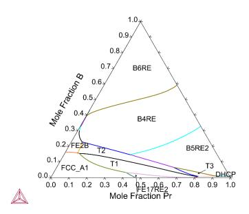
Figure 12: Calculated Fe-Pr-B liquidus projection.
