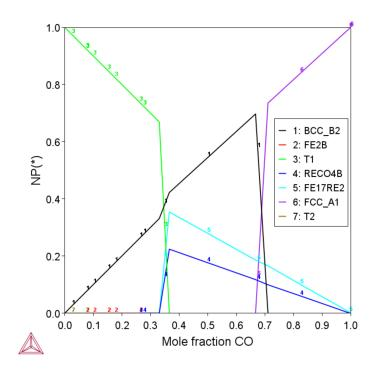
Figure 1: Calculated Ce<sub>2</sub>Fe<sub>14</sub>B-Co step diagram at 900 °C.
