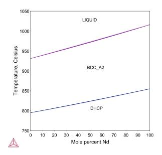
Figure 8: Calculated Nd-Pr phase diagram.
