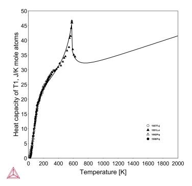
Figure 4: Calculated heat capacity of  $Nd_2Fe_{14}B$  (T1) with experimental data.
