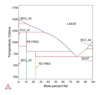
Figure 6: Calculated Fe-Nd phase diagram.
