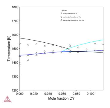
Figure 2: Calculated Nd<sub>2</sub>Fe<sub>14</sub>B-Dy<sub>2</sub>Fe<sub>14</sub>B isopleth compared with experimental data from [1989Gri].
