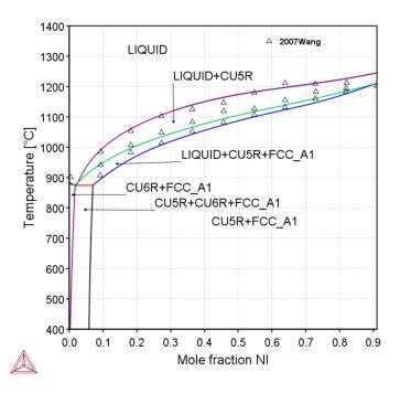
Figure 9: The calculated vertical section with 9 at.% Ce in Cu-Ce-Ni system along with the experimental data [2007Wan].
