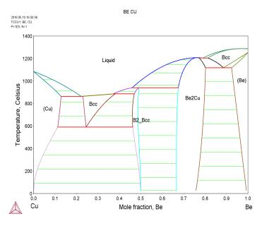
Figure 3: Calculated Cu-Be phase diagram.
