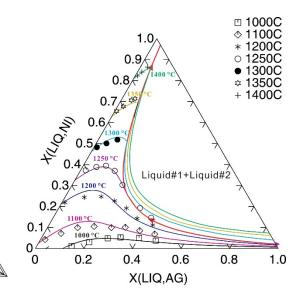
Figure 10: Calculated liquidus projection along with experimental data [199Kub] in the Cu-Ag-Ni system [2008Liu].
