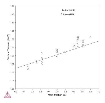
Figure 13: Surface tension of Au-Cu at 1381 K. Experimental data are taken from [2006Paj].
