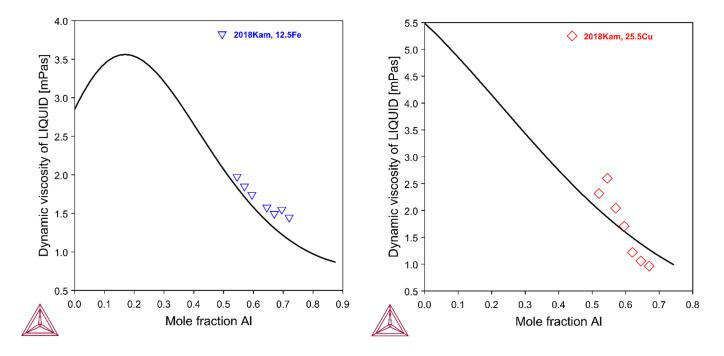
Figure 18: Kinematic viscosity of Al-Cu-Fe alloys at 12.5 at% Fe (left) and 25.5 at% Cu (right) along with experimental data from [2018Kam].
