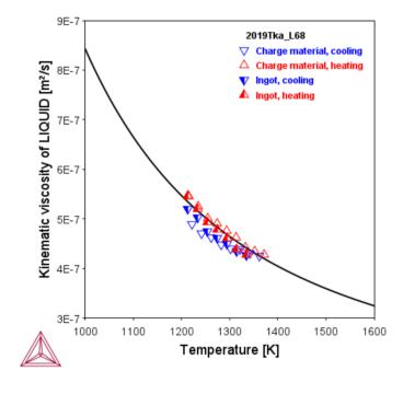
Figure 25: Calculated kinematic viscosities of the melts of L68 brass along with experimental data from [2019Tka].
