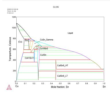
Figure 2: Calculated Cu-Sn phase diagram [2009Li].
