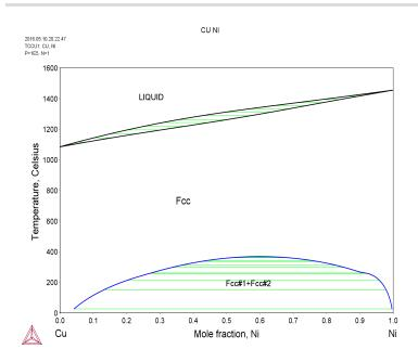
Figure 4: Calculated Cu-Ni phase diagram [1992anM].
