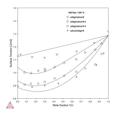
Figure 15: Calculated surface tension of Ag-Cu, Au-Cu and Ag-Au-Cu alloys at 1381 K along with experimental data from [1981Gal].
