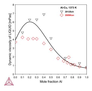
Figure 16: Calculated dynamic viscosity of Al-Cu at 1373 K along with experimental data from [2009Kon; 2012Sch].
