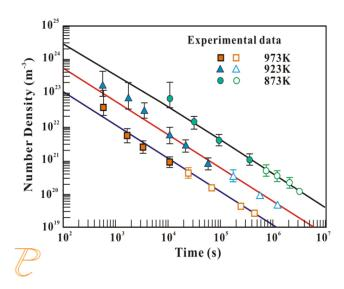
Figure 24: Simulated and experimental number density of fcc Co-Fe precipitate in Cu- 0.68 at.%Co-1.52 at.%Fe alloy annealed at 973, 923, and 873 K. The solid symbols are experimental data [2009Wat] for spherical particles; and the open symbols are for cuboid particles.
