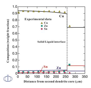
Figure 21: Calculated composition profile through half dendrite cross section in Cu-4.9wt.%Pb-5.2wt.%Sn-4.5wt.%Zn alloy during the solidification process along with experimental data [2009Kor]. The cooling rate is 0.16 °C/s.
