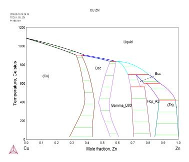
Figure 1: Calculated Cu-Zn phase diagram [2011Wan].
