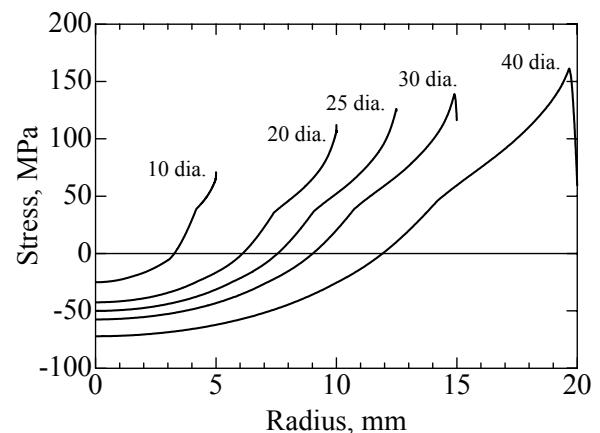
Fig. 3 Simulated Circumferential Stress Distribution in SKS3 Tool Steel Specimens
